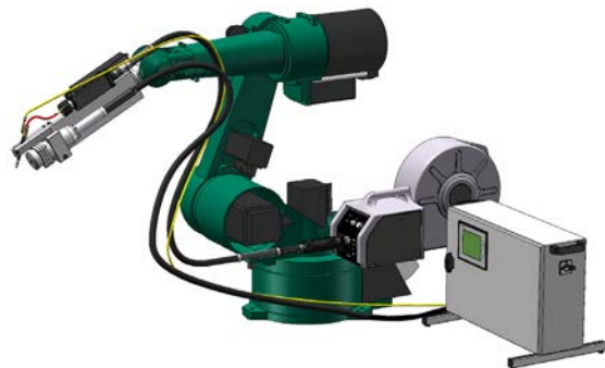
System with drive unit with torch head, control, spool holder and wire feeder application sample
